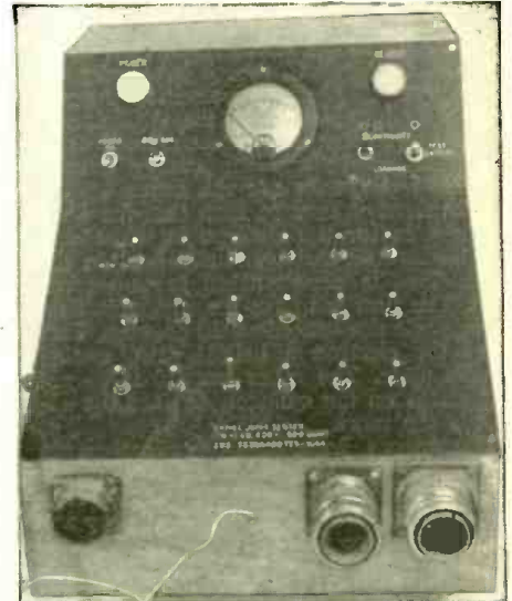
Special cables for production checking are fitted to the checker's three receptacles.
